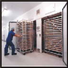
Aluminium trolleys: Light-weight and highly maneuverable
