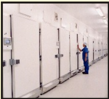
Avida setters are supplied with a raised front fascia as standard to enclose the setter room corridor and allow full control of incoming air quality and volume.
